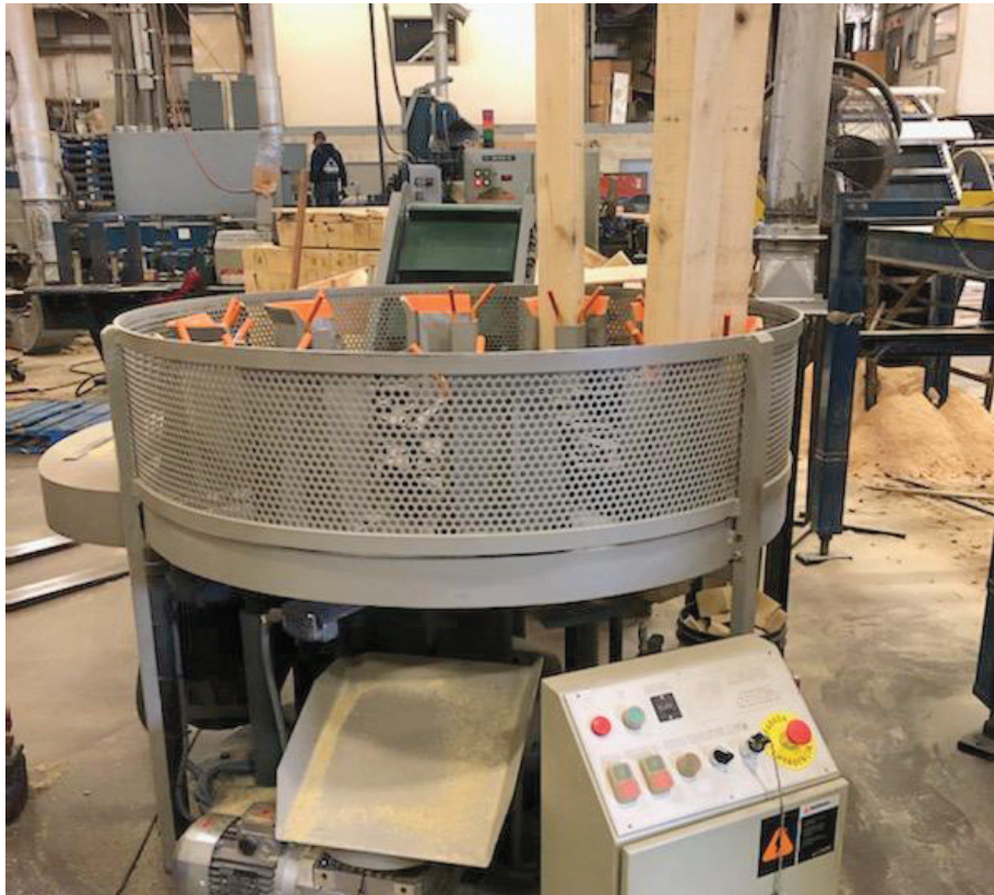
Block Cutting: In March 2019, John Rock also added a Cape block cutting machine for their expanding block pallet business. The productive carousel type block saw made an immediate impact to production after its installation.
